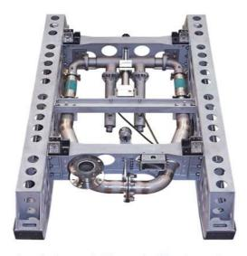
The **ACSM ROV Jetting Tool** is a simple but reliable and effective submarine cable burial tool for Post Lay Burial (PLB) operations. By means of the pressurized water from the ROV jetting pump the water flow is jetted into the seabed by a pair of legs with nozzles digging an open trench where the cable lays down in cohesive and non-cohesive soils: seabed sediments of silt and clay, fine and coarse sands and gravel, among others.
